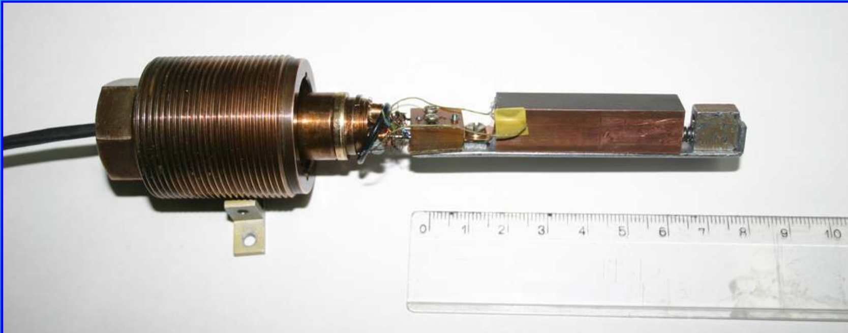
Fig.5. Love wave waveguide, Cu surface layer on a steel substrate (on the right), connected to the high-pressure lead through (on the left).
